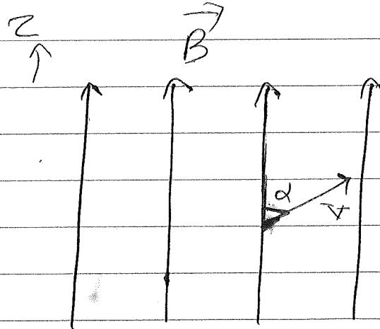
$$\frac{v_{\perp}^2}{r_{\text{gyr}}} = \frac{eBv_{\perp}}{c} \Rightarrow$$
